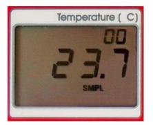
The LCD display consists of the total number of logged measurements in the upper right hand corner, the real-time temperature reading in the center, and the selected menu options along the bottom.
