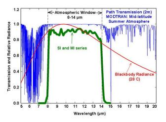
Spectral response of MI series infrared radiometers. Spectral response (green line) is determined by the germanium filter and corresponds closely to the atmospheric window of 8-14  $\mu$ m, minimizing interference from atmospheric absorption/emission bands (blue line) below 8  $\mu$ m and above 14  $\mu$ m. Typical terrestrial surfaces have temperatures that yield maximum radiation emission within the atmospheric window, as shown by the blackbody curve for a radiator at 28 C (red line).
