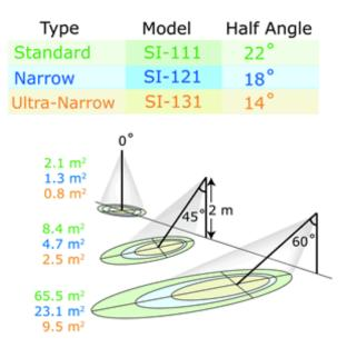
A simple FOV calculator for determining target dimensions based on infrared radiometer model, mounting height, and mounting angle, is available on the Apogee website: <u>http://www.apogeeinstruments.com/using-your-apogeeinstruments-infrared-radiometer/</u>.
