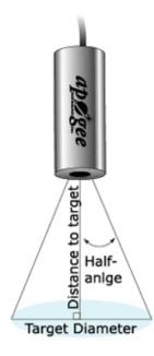
Sensor FOV, distance to target, and sensor mounting angle in relation to the target will determine target area. Different mounting geometries (distance and angle combinations) produce different target shapes and areas, as shown below.
